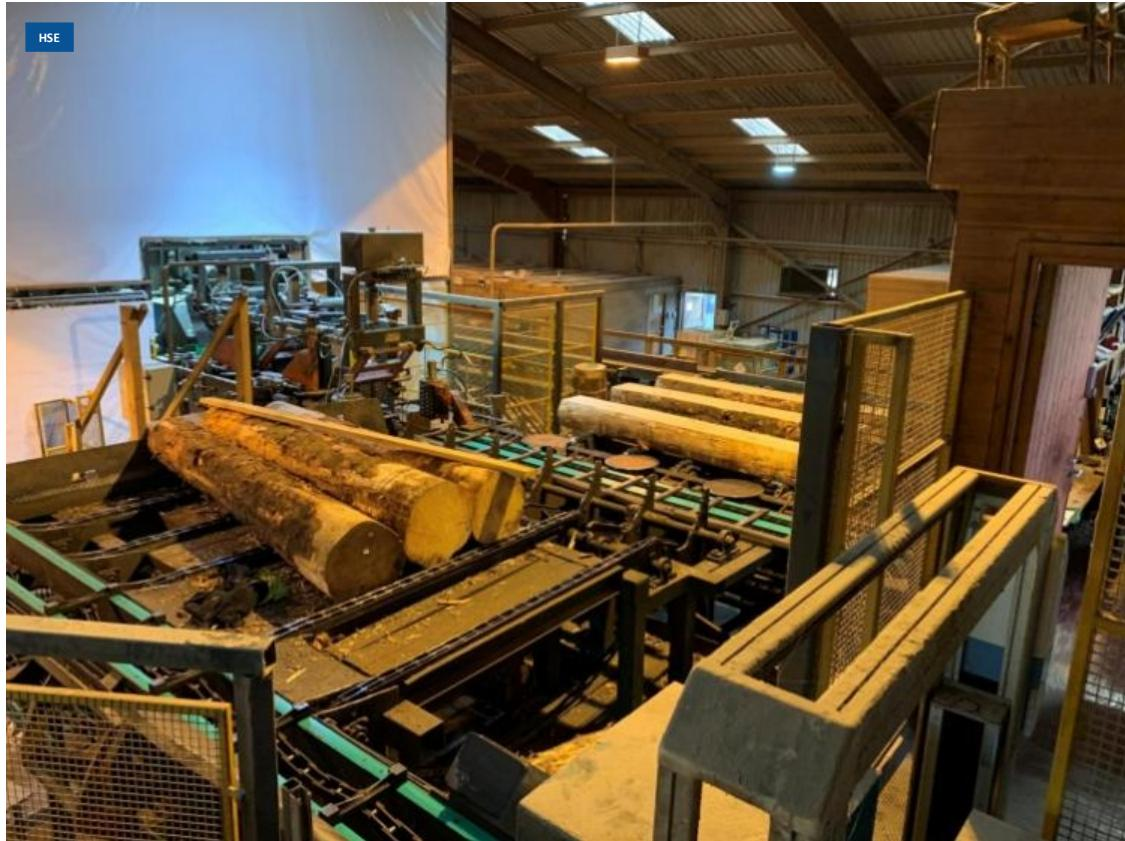
stationary conveyor bed and used a metal pole to dislodge the obstruction. While he was on the conveyor, it unexpectedly started to move, dragging his legs across moving chains and trapping them against a stop plate.
